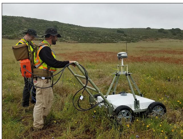
MetalMapper 2x2 static data collection
